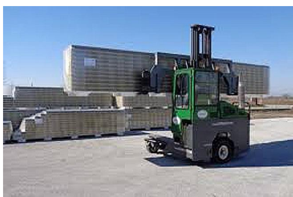
(example of unloading panels with a side forklift)
