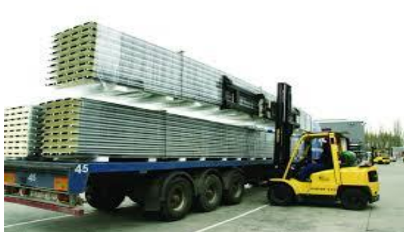
(example of unloading panels with a forklift truck)
